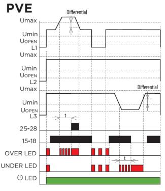
The time delay and differential trip levels help to prevent relay chatter as the monitored voltage level varies. As the relays have changeover contacts, the relay outputs can be
