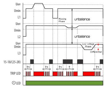
The time delay and differential trip levels help to prevent relay chatter as the monitored parameter fluctuates.
