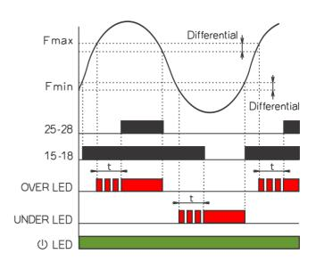
The time delay and differential trip levels help to prevent relay chatter as the monitored frequency varies.
