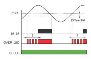
The time delay and differential trip levels help to prevent relay chatter as the monitored current level varies. As the relays have changeover contacts, the relay outputs can be inverted by wiring to the alternative terminals 15-16 or 25-26.
