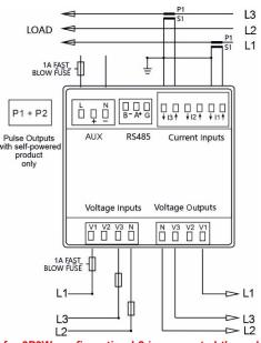
Please note for 3P3W configuration L2 is connected through the neutral and not V2.
