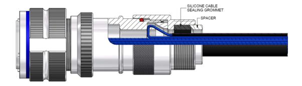
14. SCREW CABLE CLAMP NUT INTO POSITION (REFER TO ASQAW0002 FOR TORQUE GUIDELINES) AND TIGHTEN CABLE CLAMPS:
