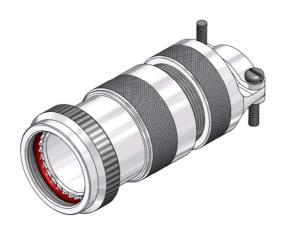
1. SLIDE THE SEPARATED CABLE CLAMP NUT, SPACER, GROMMET (THE OUTSIDE CHAMFER ON THE GROMMET FACING THE INSIDE CHAMFER ON THE SPACER), BACK CAN, GROUNDING CONES (NOTE ORDER AND ORIENTATION FROM DIAGRAM BELOW) AND BACKSHELL BODY ONTO CABLE.
