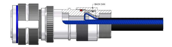
13. INSTALL CABLE SEALING GROMMET AND SPACER, AS SHOWN BELOW:
