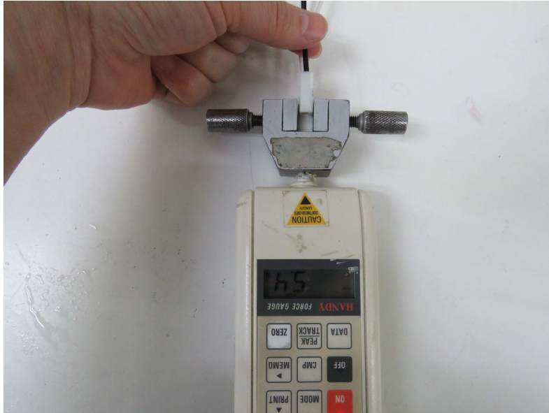
Fig. 1 Contact Insertion Force test setup
