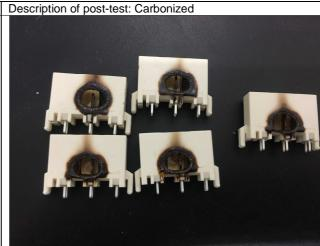
Fig.2 Test photo of post-test: A 1903415-1 (GHC 9.0 3POS HDR ASSY)
