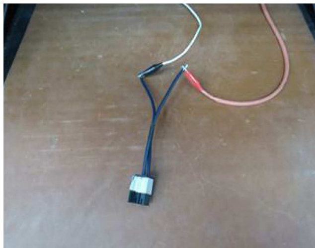
Figure 4- test setup of DWV-contact and contact
