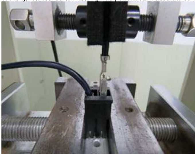
Figure 5 – typical contact insertion force setup
