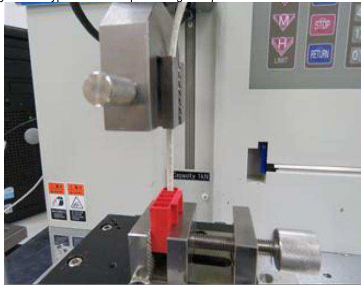
Figure 6 – typical contact insertion force setup
