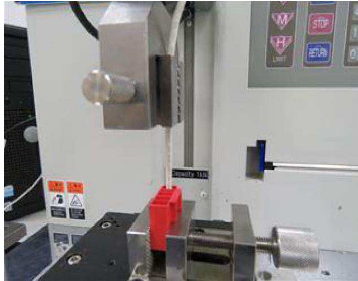
Figure – 7 typical retention force setups
