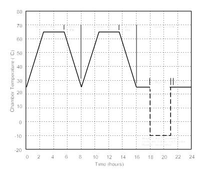
Figure 5 Humidity/Temperature Cycling Profile
