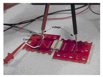
Figure 6 LLCR Measurement Points
