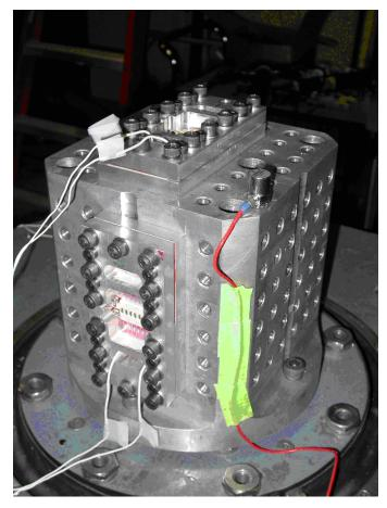
Figure 8 Vibration and Mechanical Shock Mounting Fixture
