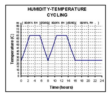
Figure 9 Typical Humidity-Temperature Cycling Profile
