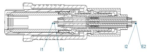
Figure 3 Low Level Contact Resistance Measurement Points
