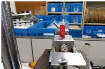
<Contact Insertion Force>
