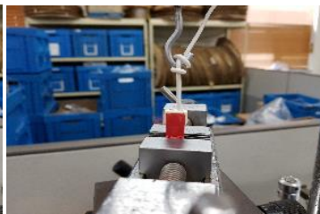
<Contact Retention Force>
