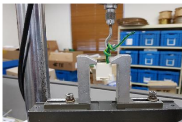
<Contact Retention Force>
