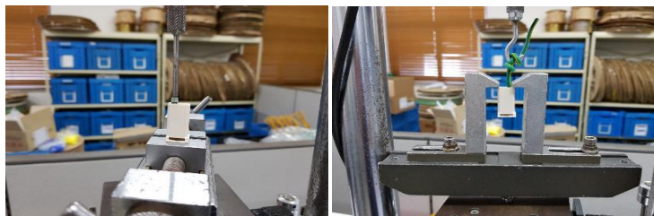
<Contact Insertion Force>
