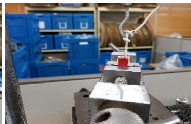
<Contact Retention Force>
