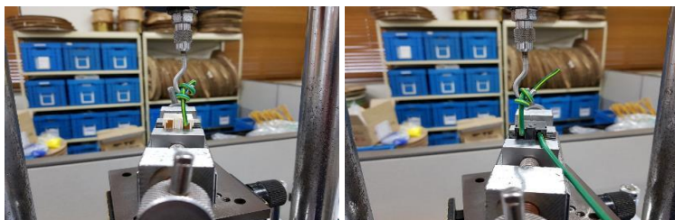
<Contact Retention Force>
