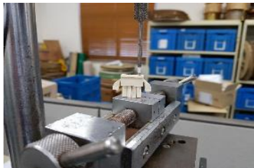
<Contact Insertion Force>
