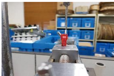
<Contact Insertion Force>
