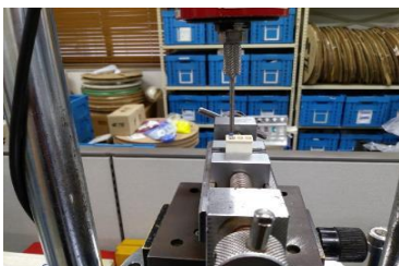
<Contact Insertion Force>
