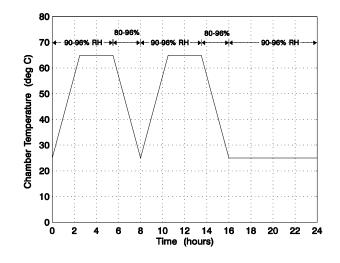
Figure 8 Typical Humidity-Temperature Cycling Profile
