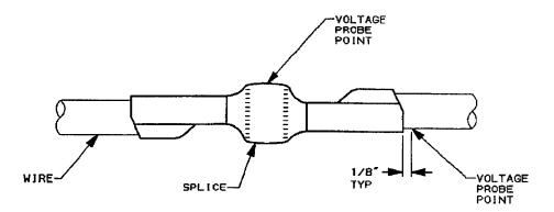
Voltage Probe Points for Splices
