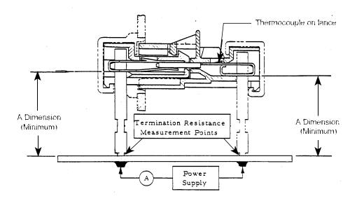
Figure 3 Typical Termination Resistance Measurement Points
