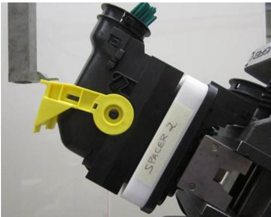
Figure 11. Mating Force Setup
