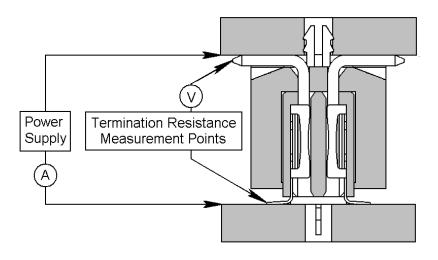
Figure 4 Termination Resistance Measurement Points
