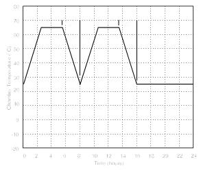
Figure 5 Humidity/Temperature Cycling Profile
