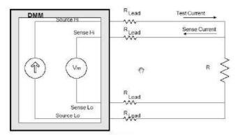
Figure 2 Termination Resistance Measurement Points
