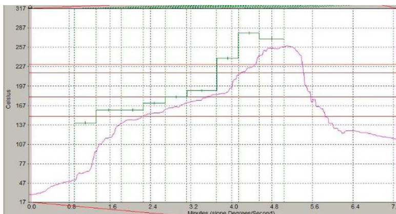
Figure 5 – Solderability Test Setup - Reflow Profile
