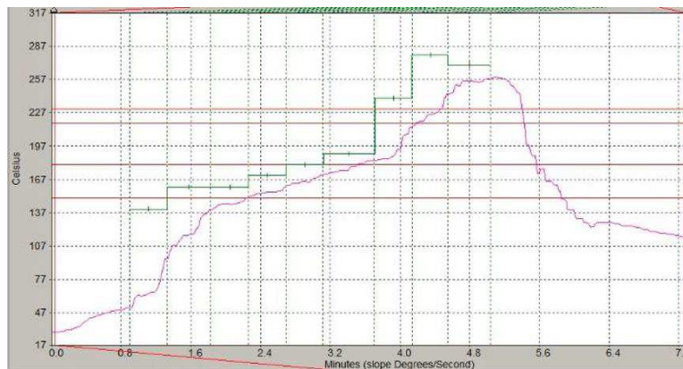
Figure 8 – Resistance to Reflow Soldering Heat – Reflow Profile
