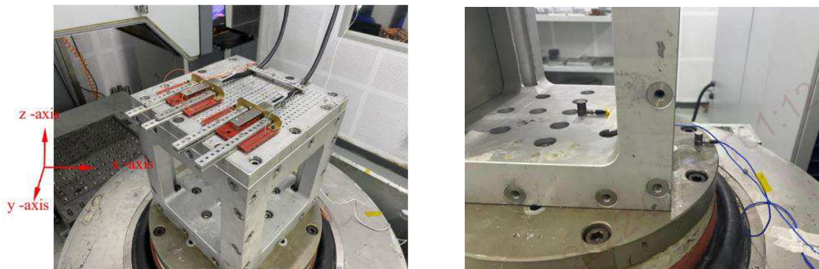
Figure 4 – Mechanical Shock Test Setup
