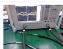
Conduct VSWR&IL&phase testing before and after the test
