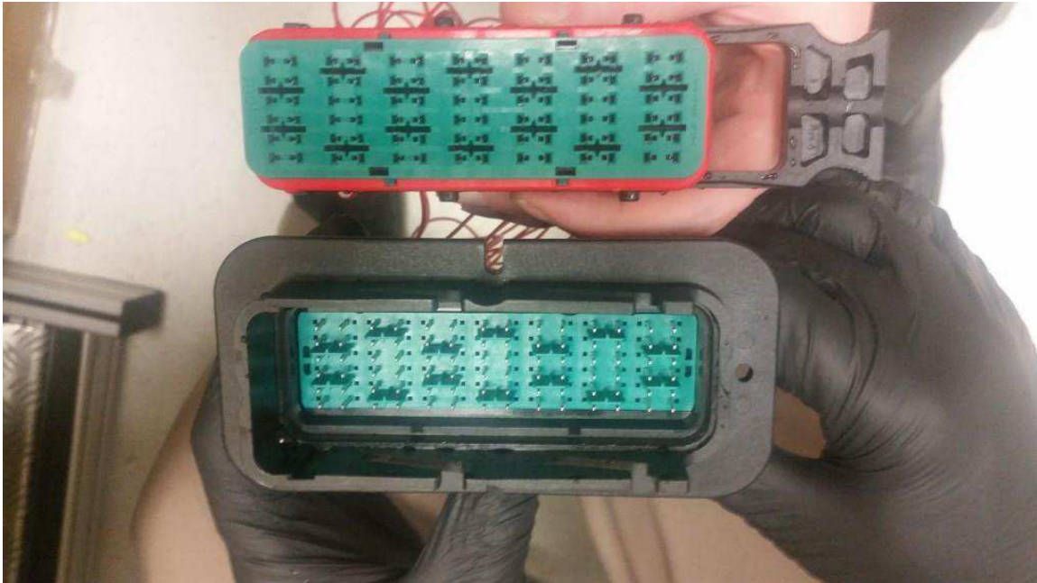
Figure 20: Visual Inspection Post Insulation Resistance/Immersion Test, No ingress of solution
