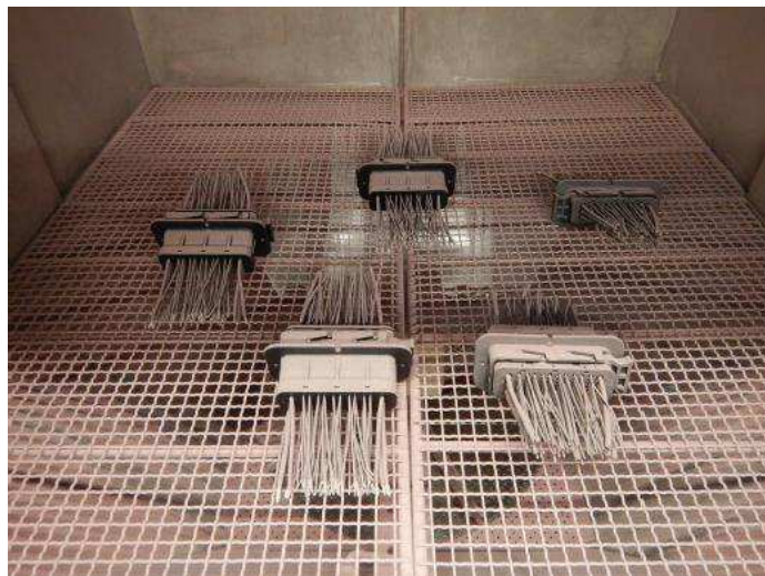
Figure 16: Specimens in the dust test chamber for IP6KX (after test)
