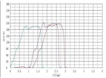
b) Test results. Meet specification 80N minimum.
