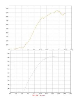
b) Test results. Meet spec: 136 N (30 lbf) minimum.
