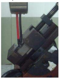
b) Test results. Meet spec: 136 N (30 lbf) minimum.
