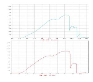
b) Test results. Meet spec: 136 N (30 lbf) minimum.
