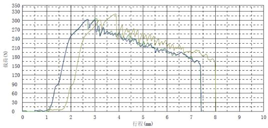
The reason for the removal tooling slide from press-fit housing. Since the size of removal tooling is limited by the room of customer's PCB. It was designed only for removal press-fit conn without lock screw. Removal force is much higher after screw locked, so the removal tooling slide.
