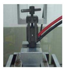
Test results: Meet specification 160N minimum.
