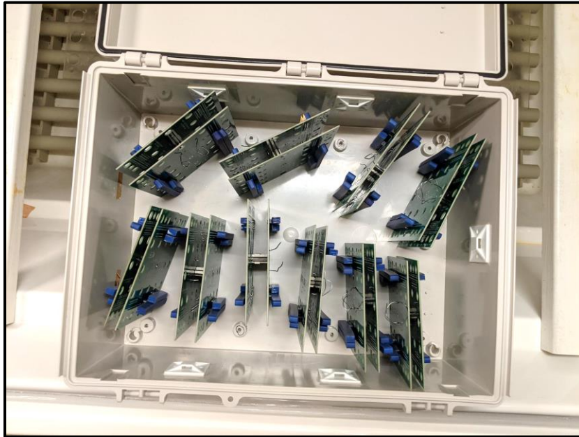
Figure 19– Test specimen in salt spray enclosure
