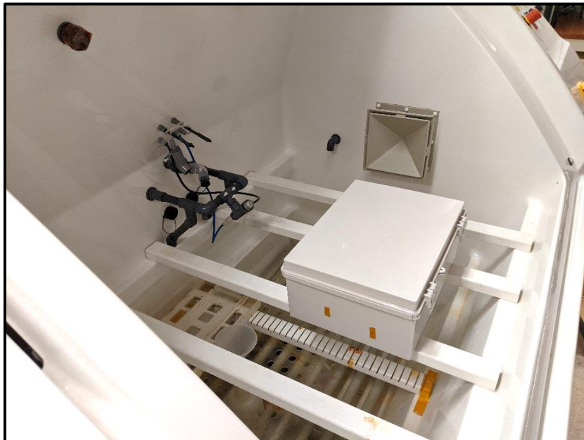
Figure 20 – Salt spray enclosure inside salt chamber
