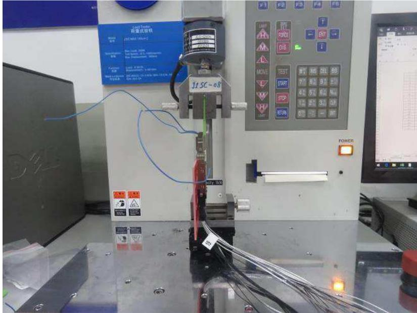
Figure 6 – Typical Unmating Force Test Setup
