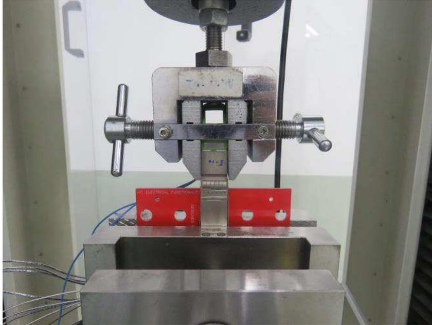
Figure 4 – Typical Cage Latch Axial Retention Test Setup
