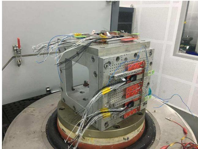
Figure 3 – Typical Random Vibration Test Setup
