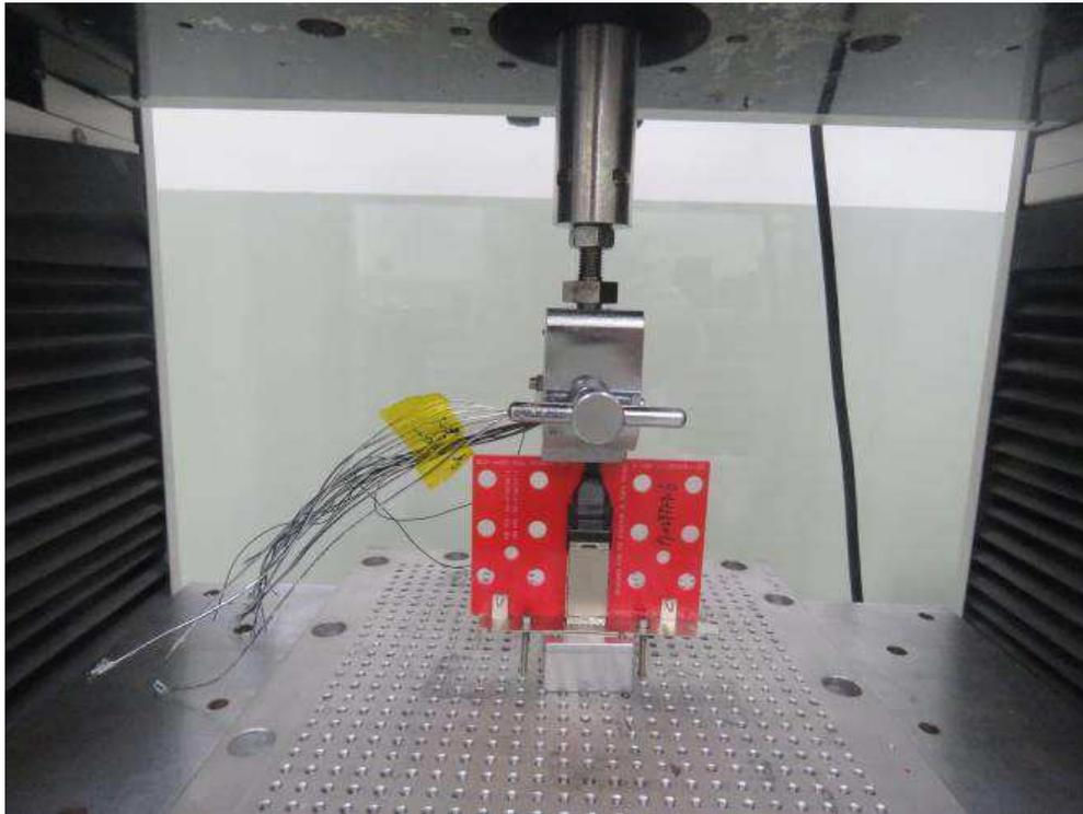
**Figure 9 – Typical Receptacle Latch Axial Retention Test setup**
