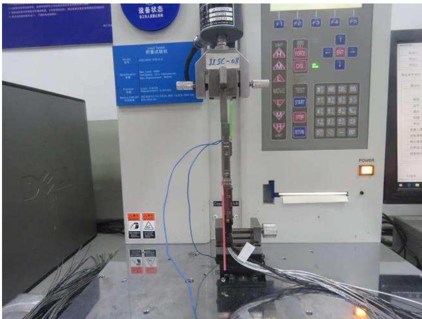
Figure 5 – Typical Mating Force Test Setup
