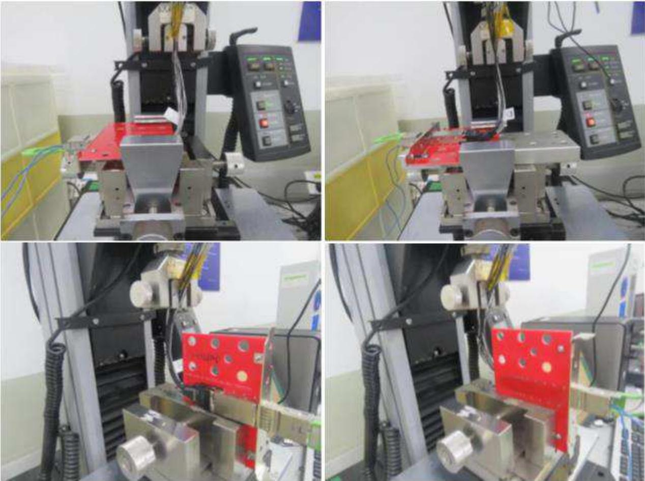
Figure 10 – Typical Receptacle Latch Lateral Retention Test Setup
