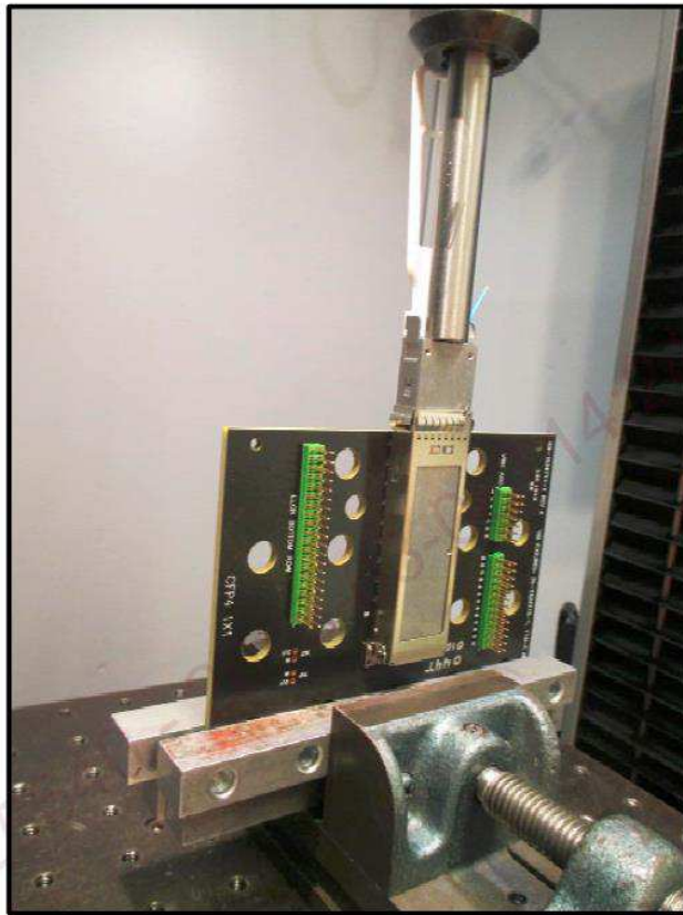
Figure 8 – Transceiver Insertion Force Test Setup
