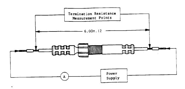
Figure 1 Typical Termination Resistance Measurement Points
