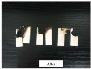
Figure 3 - visual check for GWT 750°C test
