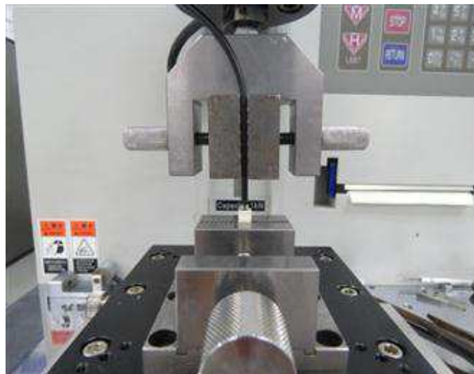
Figure 5 – typical contact insertion force setup
