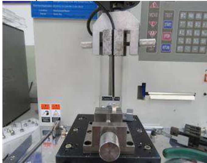
Figure – 6 typical retention force setups
