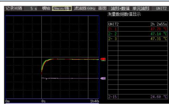
Temperature measurement photograph- Un-Shielding 4pin specimen
