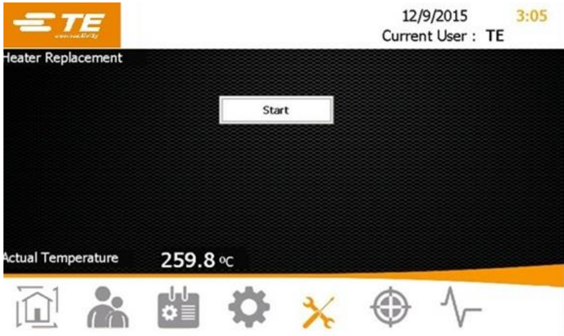
Fig. 29 : Heater Replacement display
