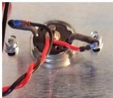
Fig. 82 : Electrical motor connections
