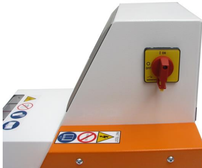
Fig. 6 : Main Switch with Emergency Stop Function
