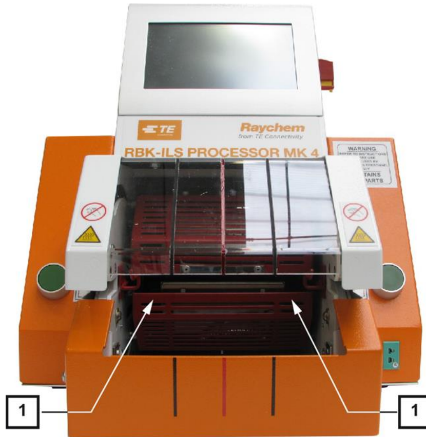
Fig. 47 : Moving the lower heating chamber manually
