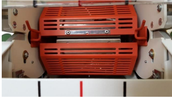
Fig. 73 : Heating chamber in the rear position
