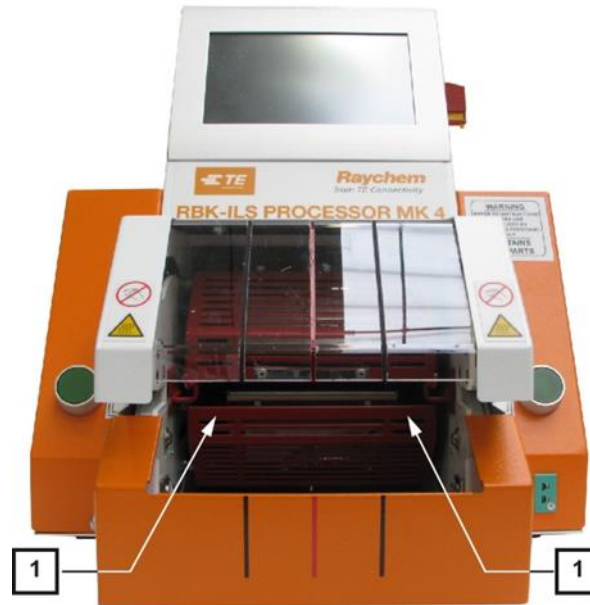
Fig. 44 : Moving the lower heating chamber manually
