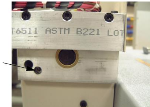
Fig. 4 : Model 19SS Heater Opening Inhibit (main upper cover removed)
