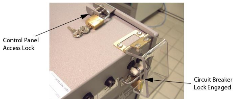
Fig. 6 : Model 19SS Circuit Breaker and Control Panel Access Locks
