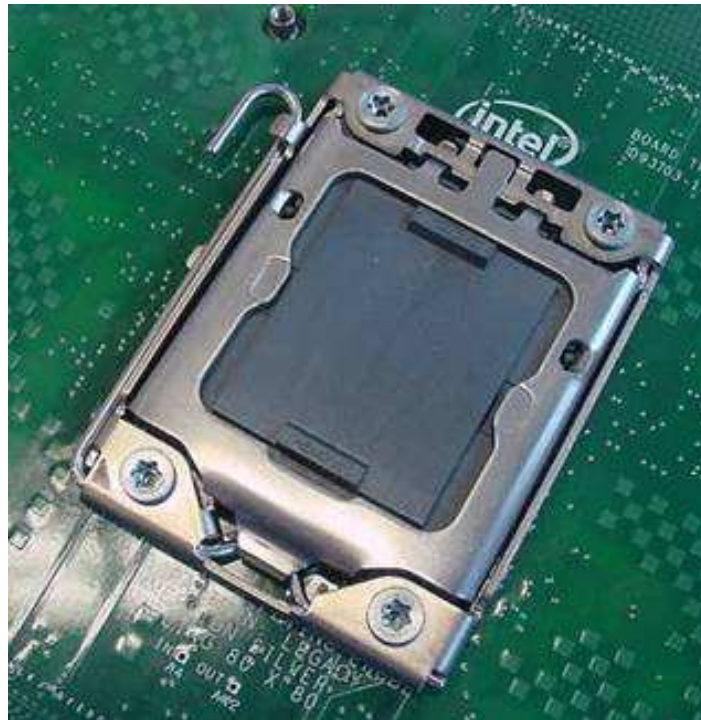
Fig.25 Completion ILM cover assembly and back plate assembly
