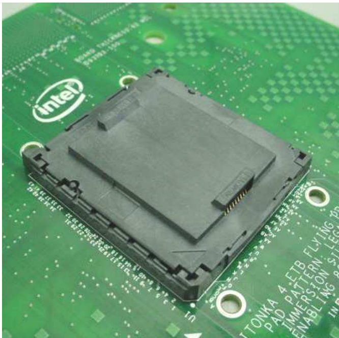
Fig.9 LGA1366 / LGA1356 socket on PCB
