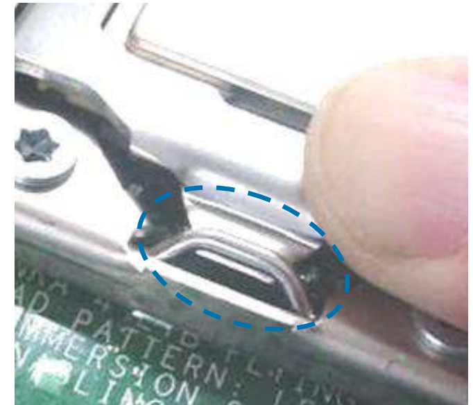
Fig.49 Confirm the lever has engaged the load plate tab
