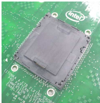
Fig.2a LGA1366 / LGA1356 socket with PnP cap (on PCB)
