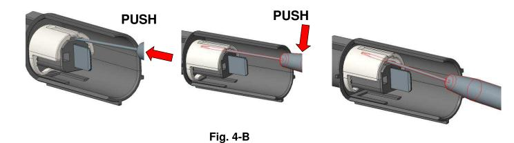
After inserting the extraction tool, pull out the wire from the housing cavity.
