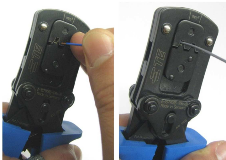
Figure 4: Insert the wire into the crimping zone (left), close the hand tool (right) (as illustrated)
