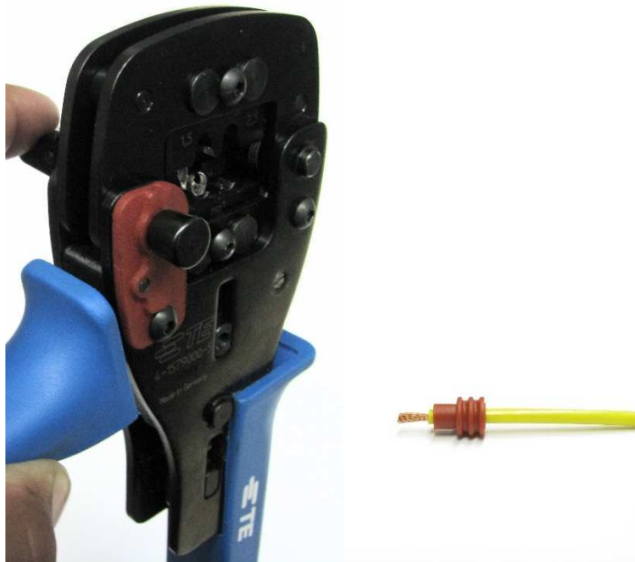
Abb. 3 : Terminal placed in the lower crimping die (left) Placing the sealing ring and wire together (wire)
