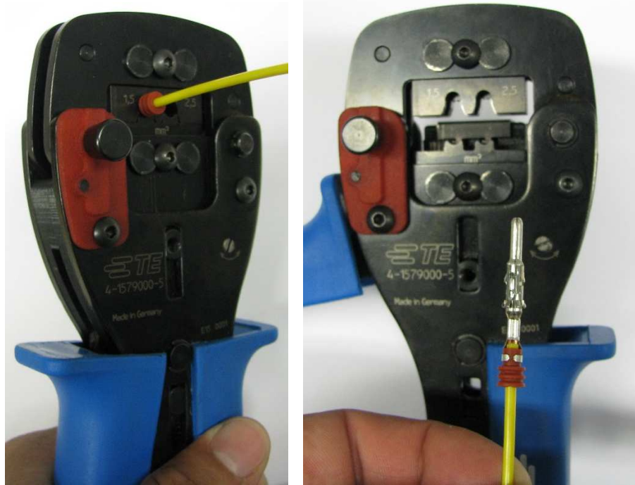
Abb. 5 : Tool handles completely closed (left), check the crimped terminals (right)
