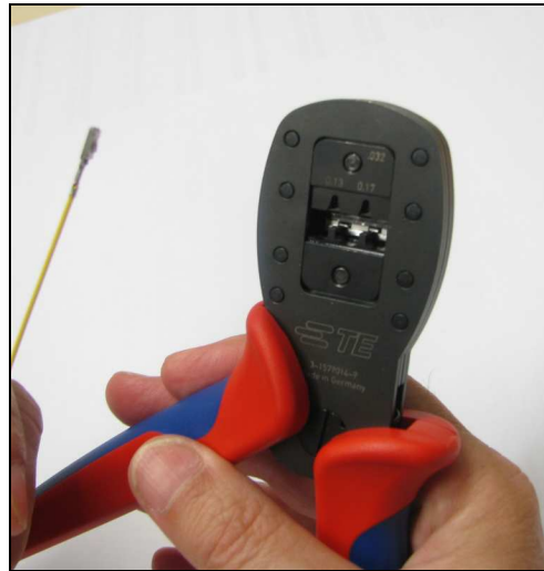
Picture 10: Checking the crimped contact
