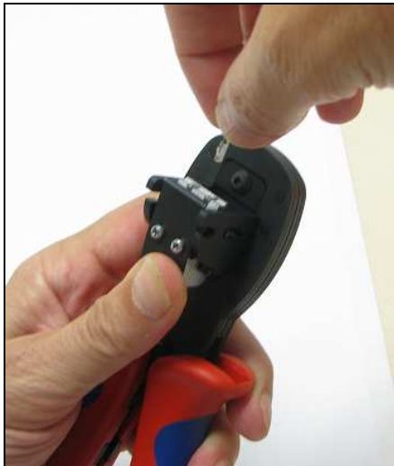
Picture 5: Inserting the contact up to stop into the contact locator
