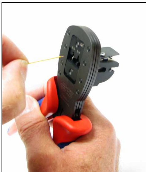
Picture 7: Inserting stripped wire in to the crimp sleeve of contact up to wire stop
