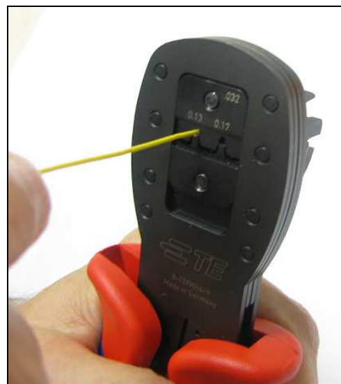
Picture 8: Squeeze handles and crimp
