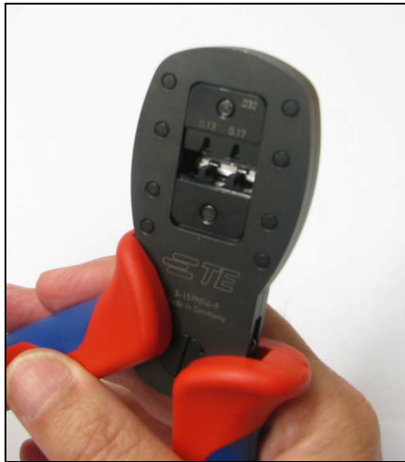
Picture 3: Let the hand tool open fully
