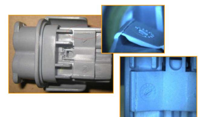
The tests were realised with these configuration. The hinge opening is possible if we need to remove the terminals to replace another on the connector. The closing is possible too.
