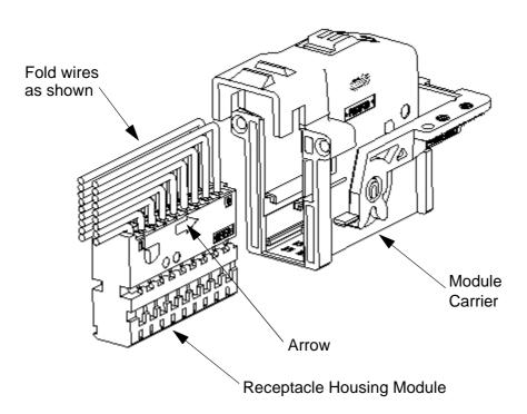
Fold the wires then insert the module with the arrow pointing towards the Module Carrier.
