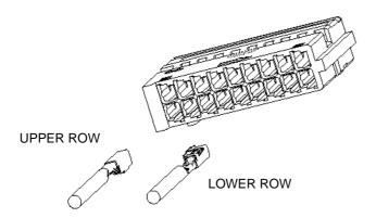
Insert the contact into the housing upper row.
