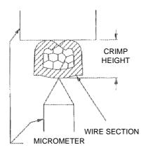
2. Special-purpose micrometer for crimping height measurement.
