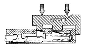
Push the tool P/N 951038-1 towards the receptacle housing module until contact is made.
