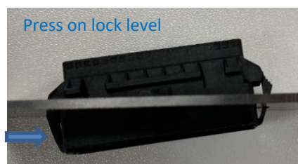
Fig 6 uninstalling tilt connector from panel
