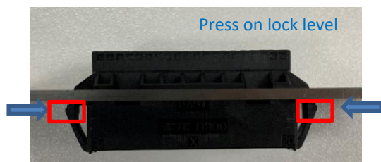
Fig 5 uninstalling connector from panel
