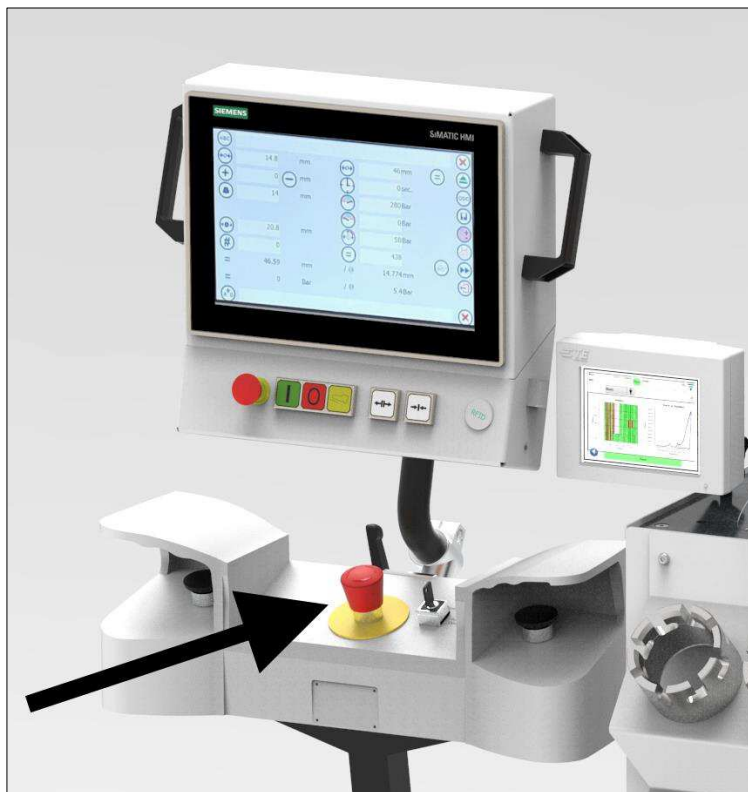
Figure 2: Emergency stop button.
