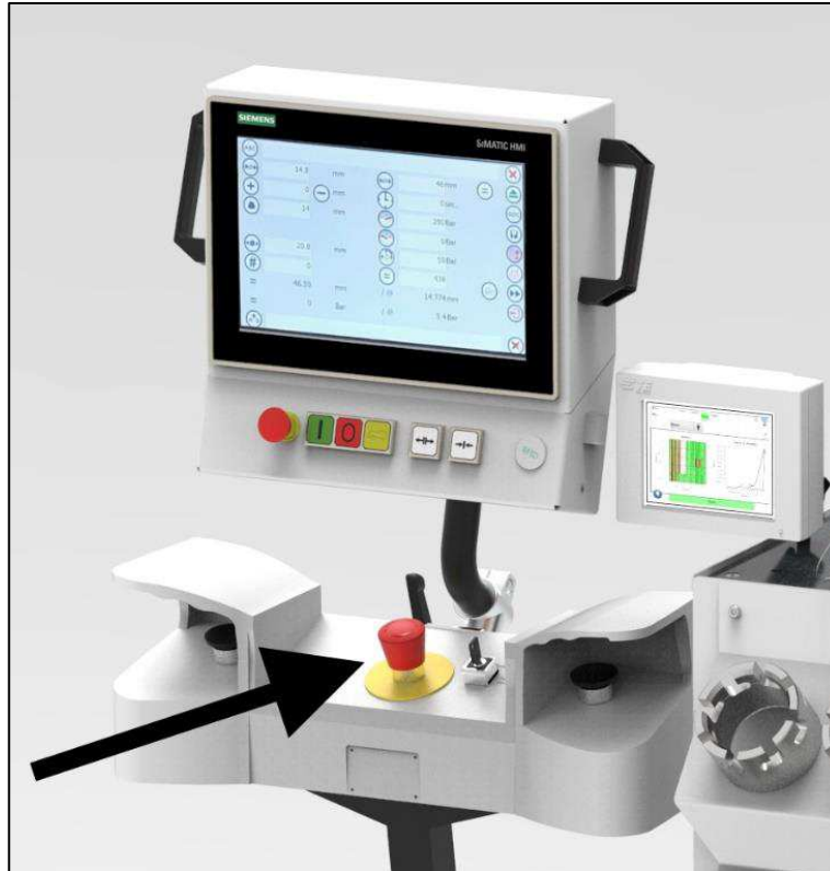
Figure 18: Emergency stop button.
