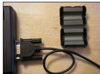
1 x ferrite core to every connection on the interfaces "one loop" as shown...
