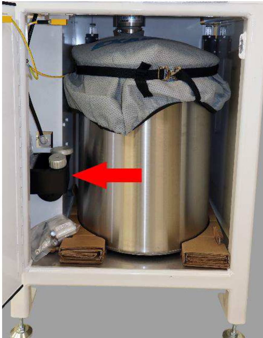
Figure 95: Location of tooling holder
