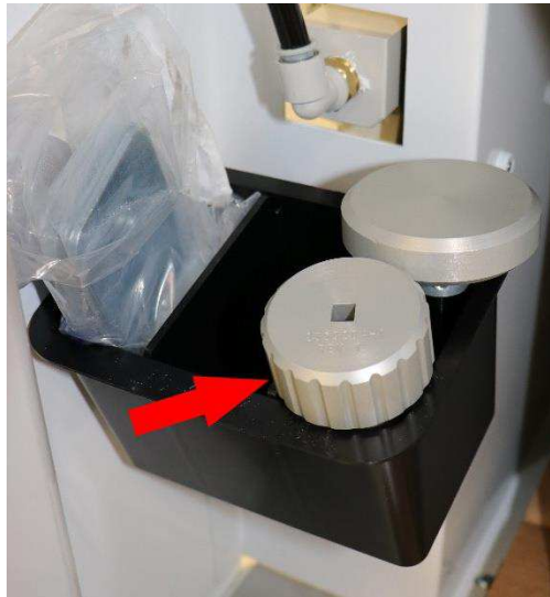
Figure 96: Mandrel changeover tool in the tooling holder
