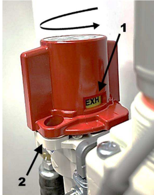
Figure 6: Main air disconnect valve in EXH position
