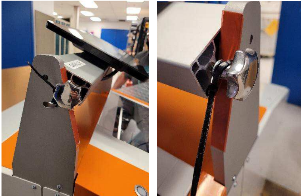
Figure 32: Removing the zip ties
