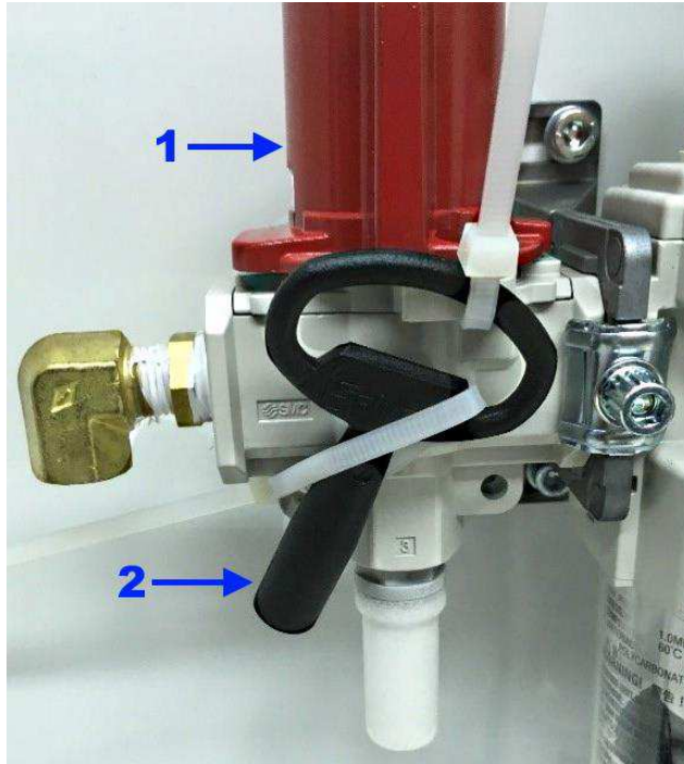
Figure 40: Electrical enclosure key and main air disconnect valve
