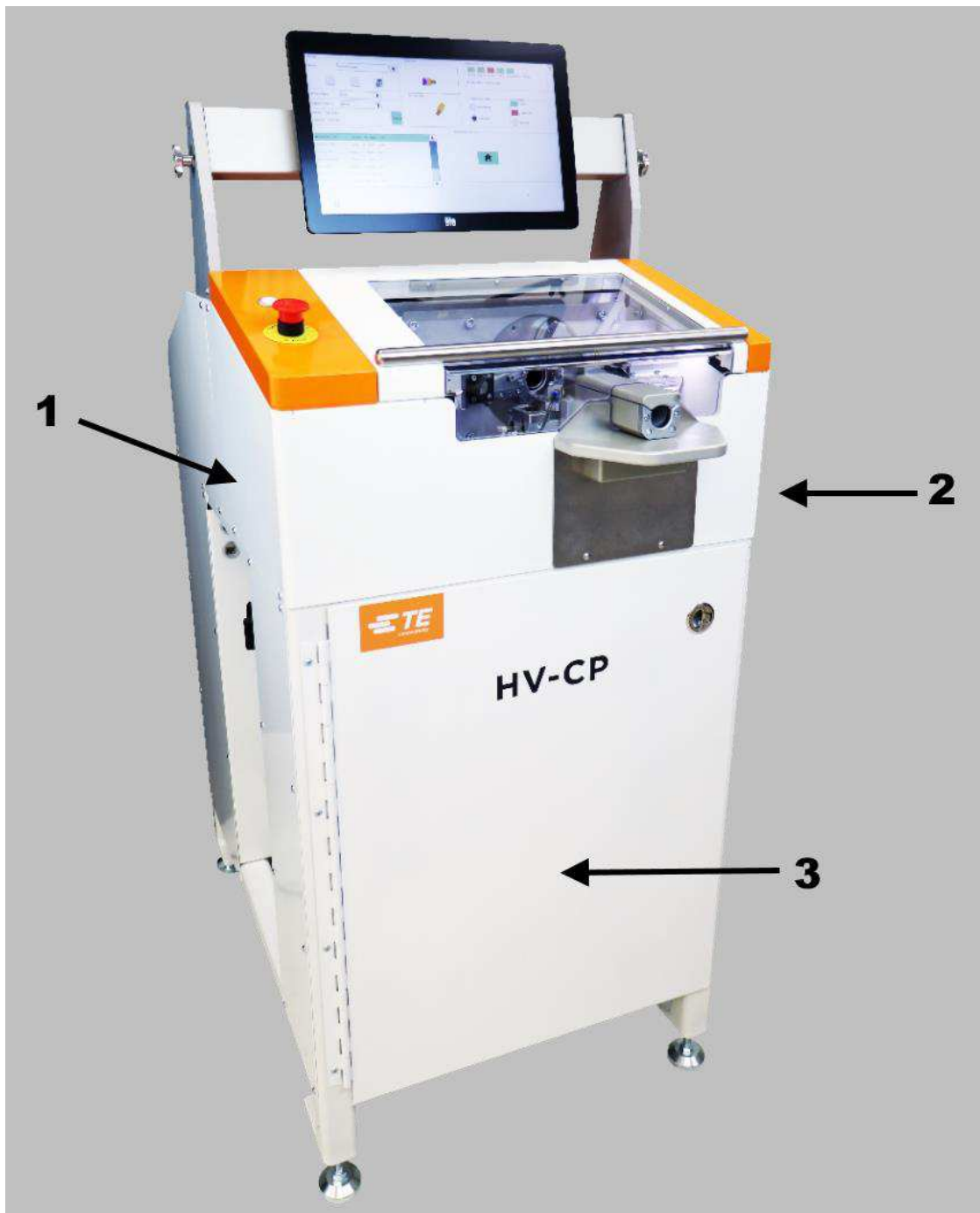
Figure 1: High Voltage Cable Preparation machine
