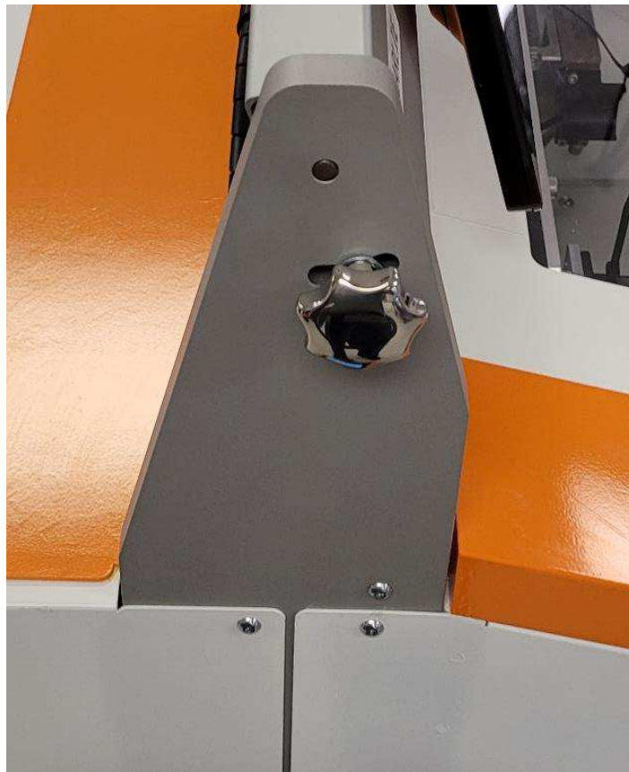
Figure 33: Reinstalling monitor adjustment knobs
