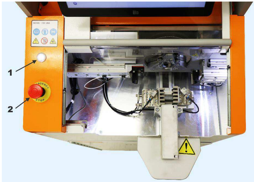
Figure 11: Emergency stop controls
