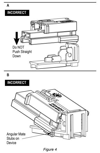
The front alignment rail design makes it more difficult to mate the connector at an angle as illustrated in Figure 4B. With enough force, it is still possible to make electric contact with the two power pins with this misalignment. However, the thumb latch will not lock onto the interface device. Most of the connector alignment to the interface is achieved through the back alignment rail design. Proper connector alignment in this area is crucial to product performance. See Figure 5.
