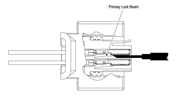
Rotate the extraction tool to release the primary lock beam while simultaneously pulling contact from rear of outer housing.
