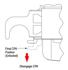
2 Unmate connector by pulling slide in direction shown.
