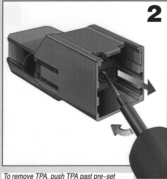
To remove TPA, push TPA past pre-set position. Use Extraction Tool 3-1579007-6 under TPA to gently pry out.
