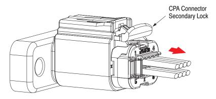
**To UNMATE:** With CPA in Position 1, DEPRESS Primary Connector Latch, then simultaneously pull connector/wires while gripping the housing with thumb, index finger, and palm (wire bundle).
