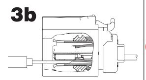
Extraction tool positioned to release beam.
