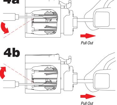
Rotate extraction tool to release beam while simultaneously pulling contact out.
