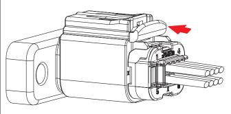
Finally, push CPA forward to engage secondary lock and ensure proper CPA locking.
