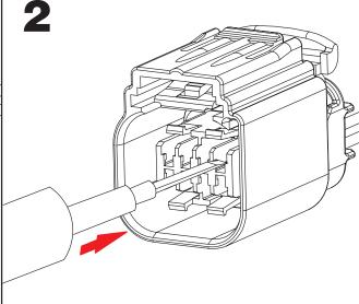
Place extraction tool under beam that holds contact in place.
