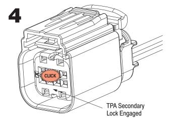
After all desired contacts are inserted, engage the TPA secondary lock. A physical resistance to fully engaging TPA indicated contact(s) is not fully inserted. Go back to Step 2.
