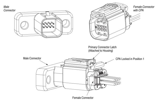
CPA is locked in Position 1 for shipping and handling before engaging the primary connector latch. CPA can not move forward or backward until the connectors are mated and the primary connector latch "clicks" and engages.
