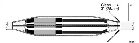
Wrap one layer of sealant around the cable jacket at the jacket cutback.
