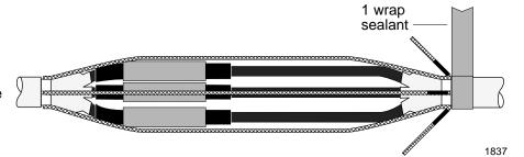
Bring the braids forward and press them into the sealant. Wrap one more layer of sealant directly over the existing sealant and ground braids.
