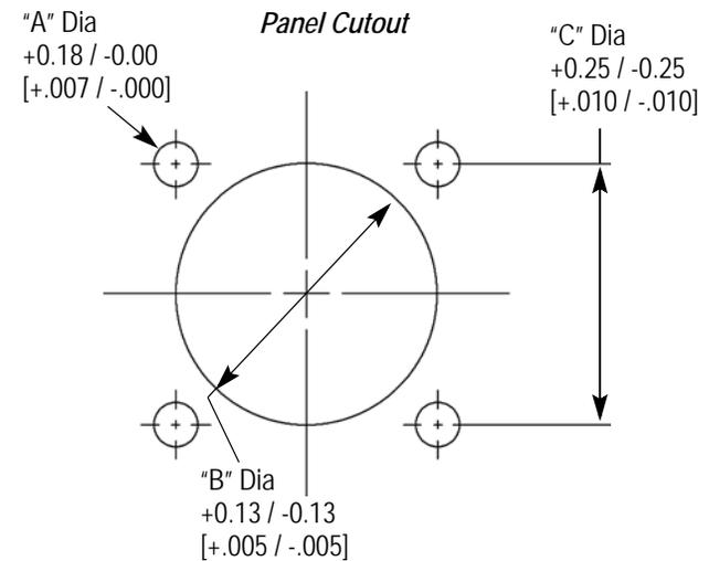
NOTE: Dimensions are in millimeters [with inches in brackets].
